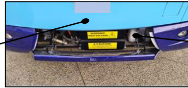
Figure 22d Filler port for windscreen washer fluid
