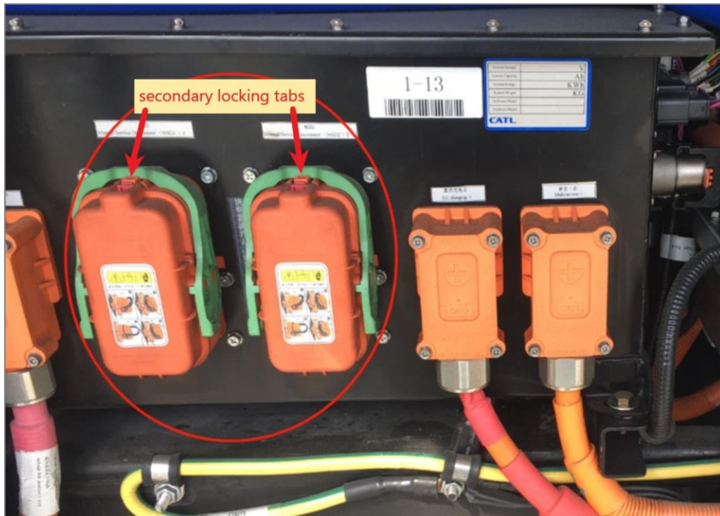
Figure 3 – S-Box MSD locking tabs and levers
